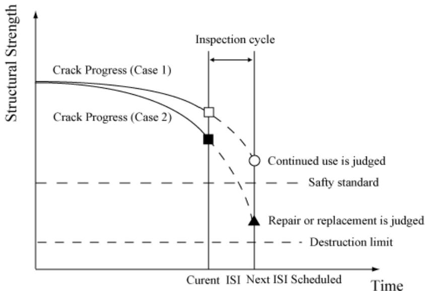
Fig. 2 Illustration of structured integrity evaluation
