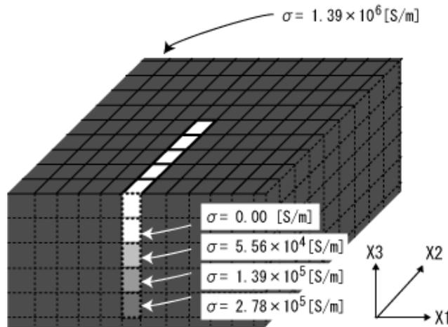
Fig. 4. Modeling of stress corrosion crack in finite element analysis
