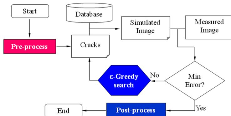
Fig. 5 Flow chart of crack shape recovery
