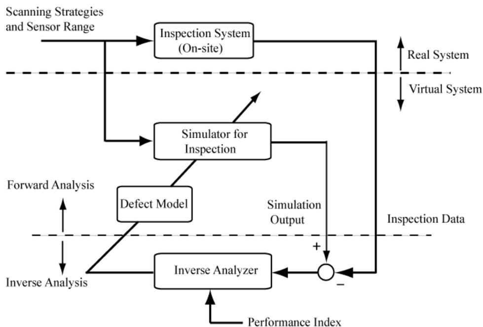
Fig. 3 Overall configuration of model based diagnosis system
