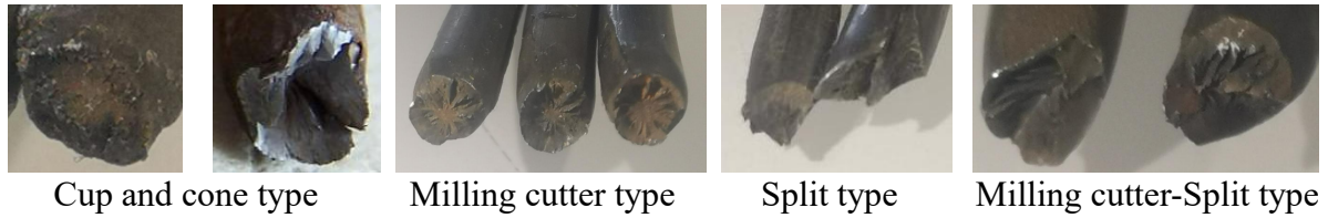
Fig. 2.10 Fracture type of corroded steel wires
