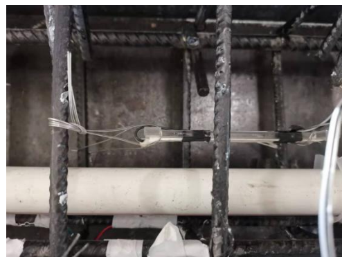
(a) 'I' plastic plate with concrete strain gage (b) Install in reinforcement cage
