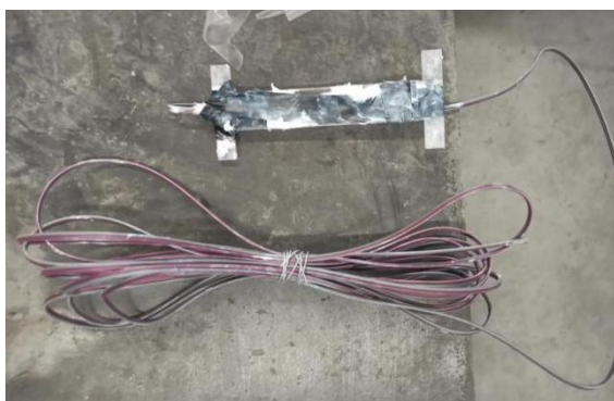
(a) 'I' plastic plate with concrete strain gage (b) Install in reinforcement cage
