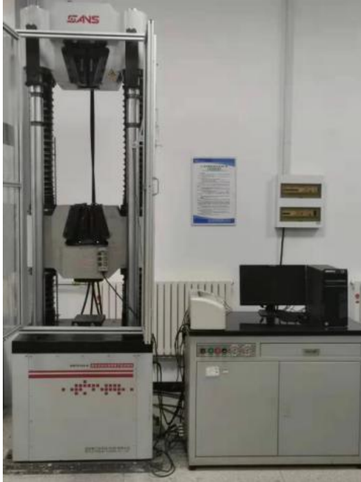
Fig. 2.6 SHT4106G microcomputer control electro-hydraulic servo universal testing machine
