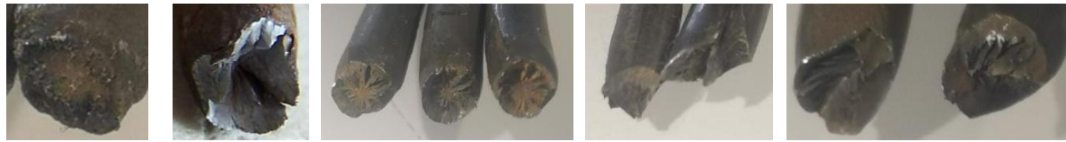
Cup and cone type Milling cutter type Split type Milling cutter-Split type
