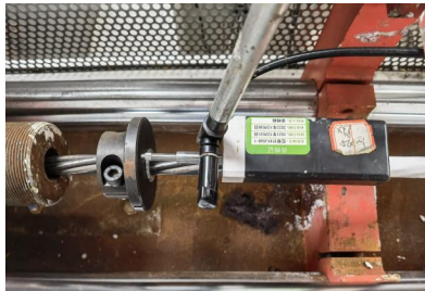
Fig. 2.21 Steel plate and displacement transducer
