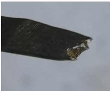
Fig 6.4 F-B-12 wire fracture type
