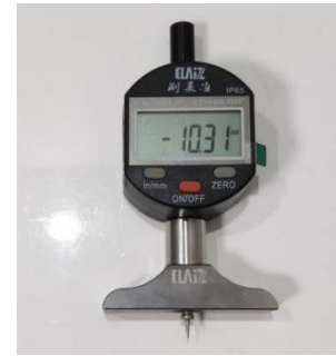
Fig. 2.25 Depth measuring instrument
