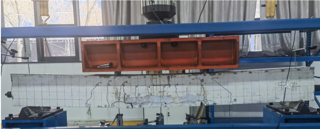
Fig. 6.2 Static loading test
