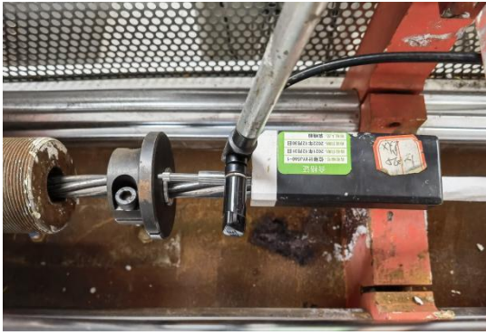
Fig. 2.4 Steel plate and displacement sensor
