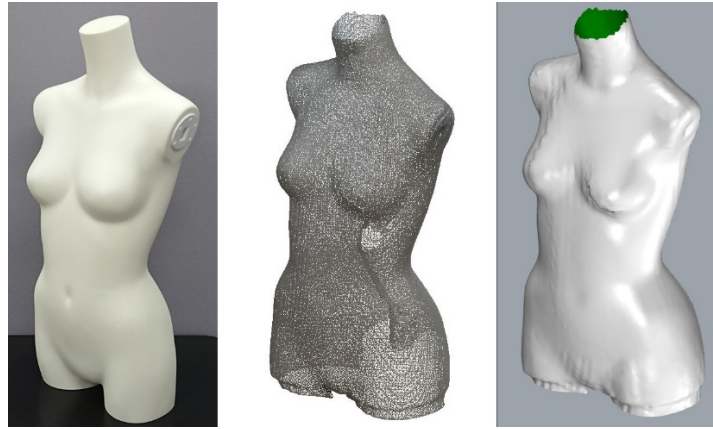
Fig.1. Original item (left), scanned mesh data (center) and shaded view by 3D CAD (right)
