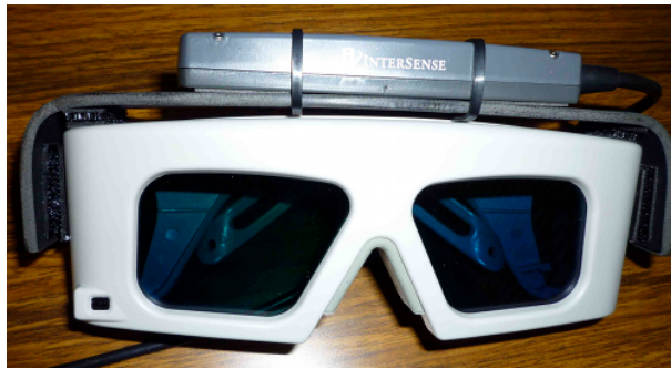
Fig. 13: Liquid crystal shutter glasses for pCAVE. Shutter switches using liquid crystal are used for the stereo view.
