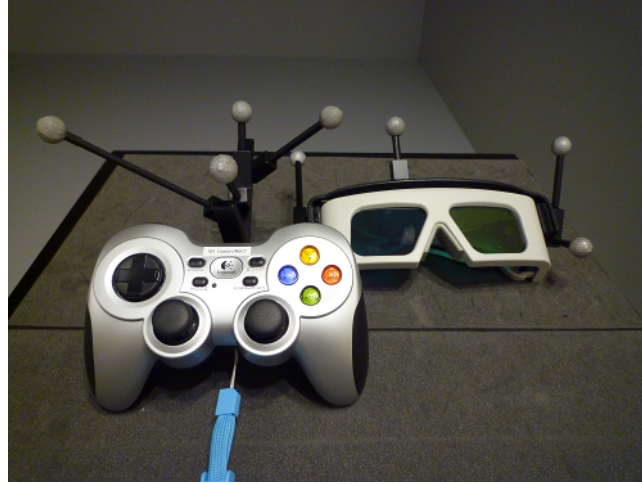
Fig. 15: Portable controller and stereo shutter glasses of \pi -CAVE. For small balls are attached each devices for the optical tracking system.
