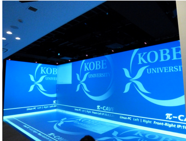
Fig. 16: An overview of \pi -CAVE system. Stereo images are projected on the four(front, right, and left walls, and the floor) screens.
