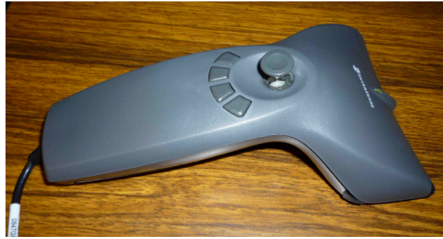
Fig. 14: Wand, a potable controller for pCAVE. There are five buttons and one joy-stick.
