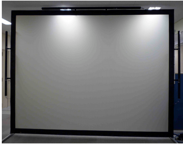
Fig. 12: The screen of pCAVE system on which stereoscopic images are projected from behind. The height is 2.6m.
