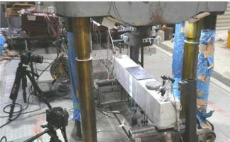
2000kN universal loading machine which is one of the equipments in our structural laboratory can conduct a compressive, tensile or bending test for construction materials from element size to full scale of the structural member.
