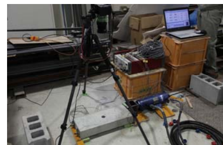
Concrete strain measurement by using image analysis
