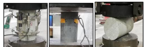
Compressive Test Tensile Splitting Fig. 2 Material tests
