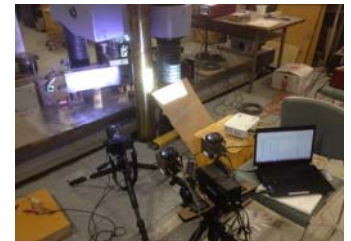
Loading test of UFC beam
